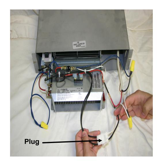
Attach the BLACK wire from the plug to the RED wire from the thermostat.
